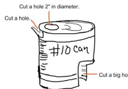
Make a calorimeter out of a #10 can and a smaller can.
